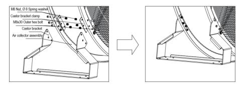
Attention: The castor bracket shall be installed symmetrically on both sides and the bottom on both sides shall be horizontal.
