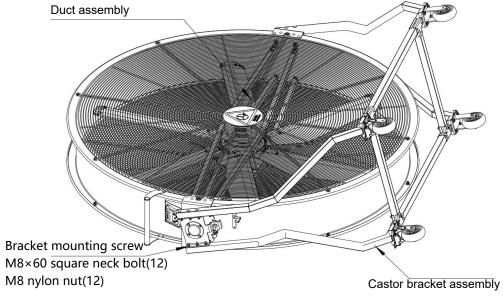
3.Adjust the angle by 45° front and rear (horizontal blowing angle 0°). There are total of 7 gears with 15° each gear.
