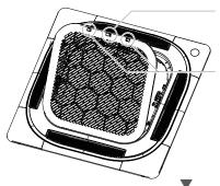
1: Open the screw cover and twist out the screw.
