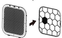
Separate the frame from the filter assembly.
