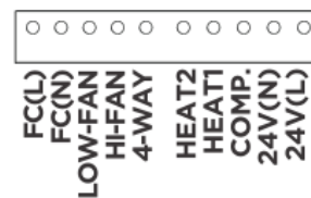
Terminal of PTAC Wall Thermostat (MODE B)
