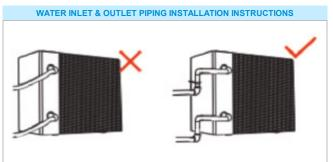
\*The pool heat pump must be connected using PVC pipes, the use of soft, flexible pipes is not recommended as the weight of these pipes will damage the internals of the unit.
