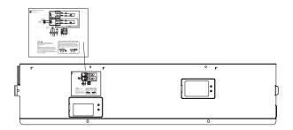
Paste the wire terminal label on the control box.
