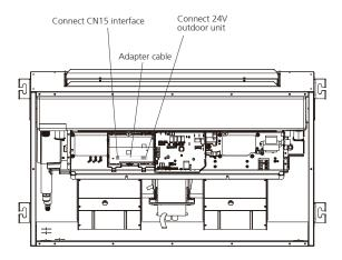
Note: The adapter cable must be used when the full 24V communication scheme is applied. That will stop the operation of outdoor for safety if the refrigerant leakage happen.
