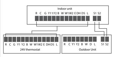
When using a 24V thermostat, please refer to the non-communicating wiring diagrams that follow:
