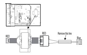
Step 5: Take the 24V transformer connection wire out from the accessory package. Connect the red connector of the transformer to the white connector and the blue connector to the control board CN12.
