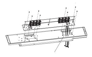
Thread wires through this hole, then install the electric heating assembly to the electric control box.
