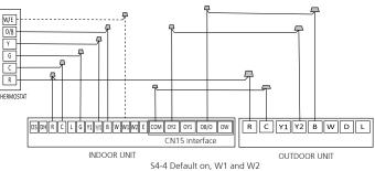
S4-4 Default on, W1 and W2 shorted for single stage Aux heat operation. Turn off to separate stages.
