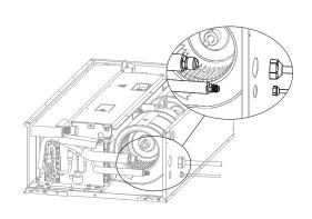
**Step 9: Connect the drainpipe**
