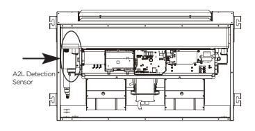
The A2L Detection Sensor is attached to a wiring harness that connects the sensor to the control board.
