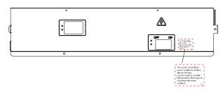
Paste the supplementary heater kit wiring diagram on the control box cover inside .
