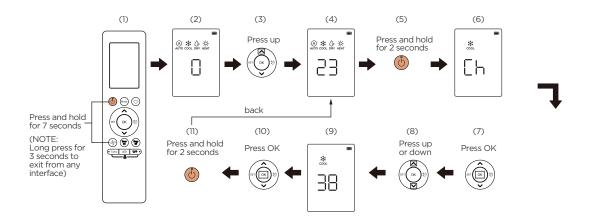
2) In engineering mode, when the number code is 25, long press "On/Off" key for 2 seconds to enter the air volume adjustment dialling code setting for heating, display Ch, press "OK" key to query the air volume adjustment value for heating, and then press "Up" and "Down" key to select the air volume adjustment dialling code for heating, and then press "OK" key, long press "On/Off" key for 2 seconds to exit. Then press "OK" key; long press 2 seconds "on/off" key to exit.
