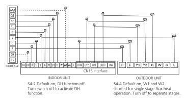
• Wiring for 2H and 2C thermostat
