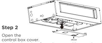
(Unplug the wires from the control box so that you can remove the control box cover.)
