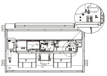
NOTE: The fixing port for the armored wire needs to be fitted to the knock-out hole on the electrical control box for protection of the leads from scratching.
