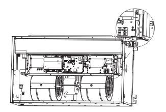
**Step 7: Install the control box cover**
