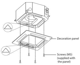
After installing the decoration panel, ensure that there is no space between the unit body and decoration panel. Otherwise air may leak through the gap and cause dewdrop. (See figure below)
