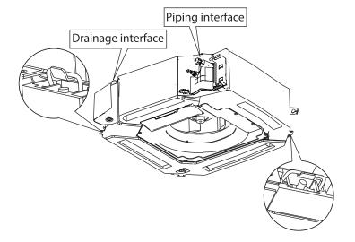
**NOTE:** If the height of the indoor unit needs to be adjusted, you can do so through the openings at the panel's four corners. Make sure that the internal wiring and drainpipe are not affected by this adjustment.
