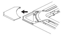
Adjust the panel by turning it to the arrowed direction so that the ceiling opening is completely covered.
