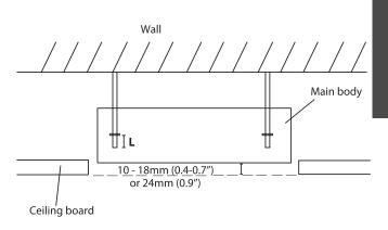
**NOTE:** The bottom of the unit should be 10-25mm(0.4-0.98") higher than the ceiling board. Generally, L (indicated in the following figure) should be half the length of the suspension bolt or long enough to prevent the nuts from coming off.
