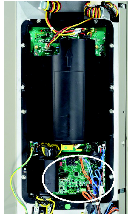
Fig. 17 - AOC (Application Operational Control) Board
