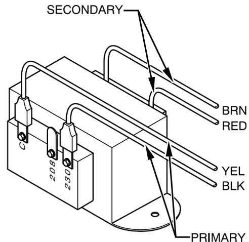
**Fig. 5 – Connection of Transformer**
