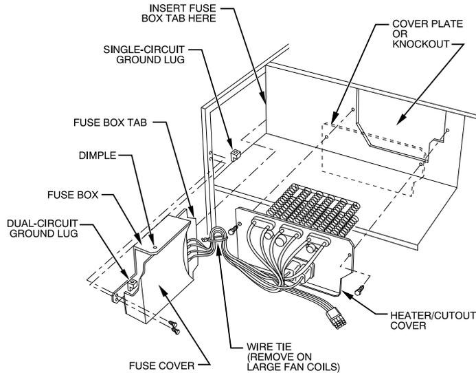
**Fig. 2 – Installation of Fused Model Heater**
