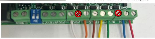
Up close view of 24 volt terminal strip on air handler. Please note which connections are used. Specifically please note that L & W are skipped.
