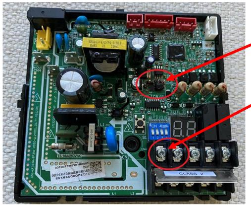
Board will burn out here if 24 volts is connected to S1 & S2.
