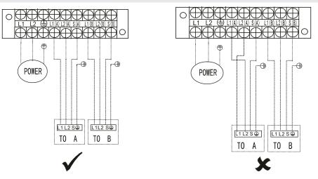
**NOTE:**Refer to the following figures if end-users wish to perform their own wiring. Run the main power cord through the lower line-outlet of the cord clamp. ---- This symbol indicates field wiring.
