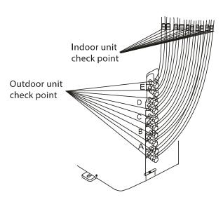
A, B,C,D are points for one-four type. A, B,C,D, and E are points for the one-five type.
