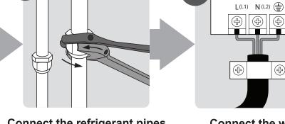
**Connect the refrigerant pipes**
