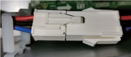
Fig. 28 — Insert the white plug wire
