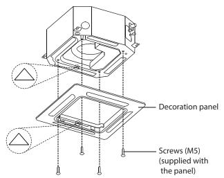
After installing the decoration panel, ensure that there is no space between the unit body and decoration panel. Otherwise air may leak through the gap and cause dewdrop. (See figure below)
