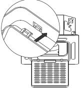
Step 4: Connect the 2 wires of the decoration panel to the mainboard of the unit.
