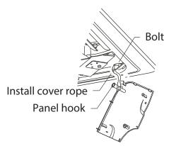
Re-installed into the style grid. Reinstall the installation cover. Fix the installation cover plate rope to the pillar of the installation cover plate, and gently press the installation cover plate into the panel.
