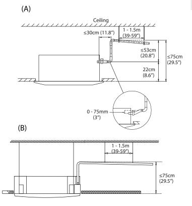
**NOTE:** When connecting multiple drainpipes, install the pipes as illustrated in the following Figure.
