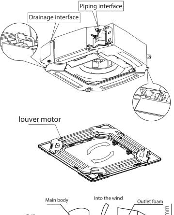
Step 2: Remove the installation covers at the four corners by sliding them outwards.
