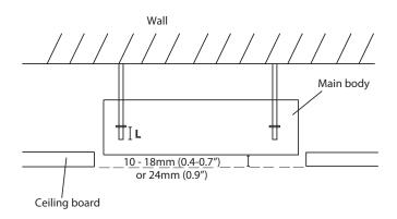
**NOTE:** The bottom of the unit should be 10-25mm(0.4-0.98")higher than the ceiling board. Generally, L (indicated in the following figure) should be half the length of the suspension bolt or long enough to prevent the nuts from coming off.
