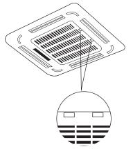
Step 2: Remove the installation covers at the four corners by sliding them outwards.
