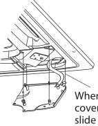
When installing the cover, slide the four slide fasteners into the corresponding slots on the panel.
