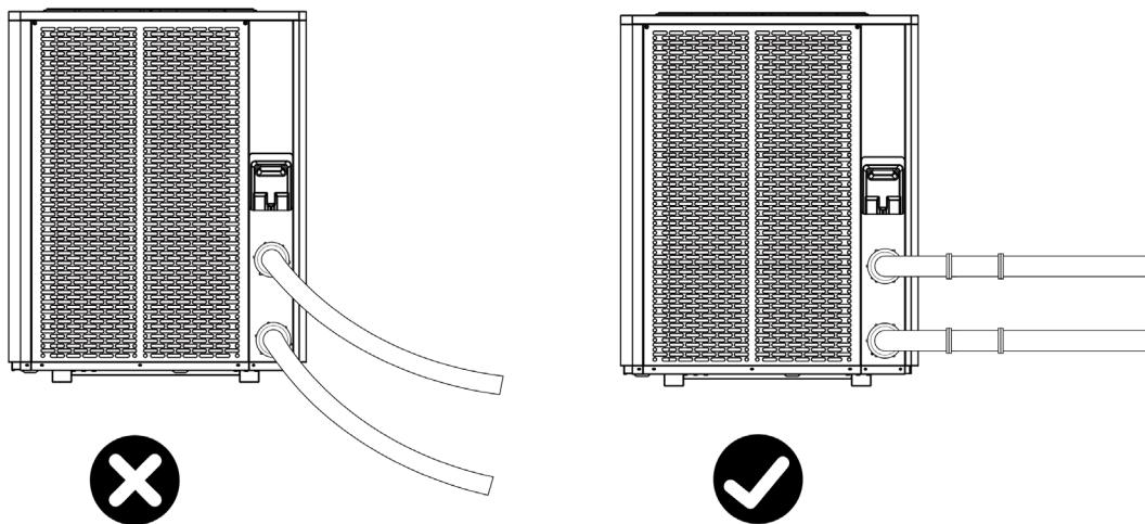
2. In order to guarantee the heating efficiency, the water pipe length should be  $\leq 10\text{m}$  between the pool and the heat pump.
