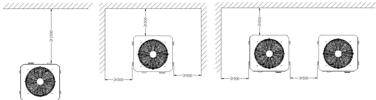
Do not put anything less than one meter in front of the heat pump.
