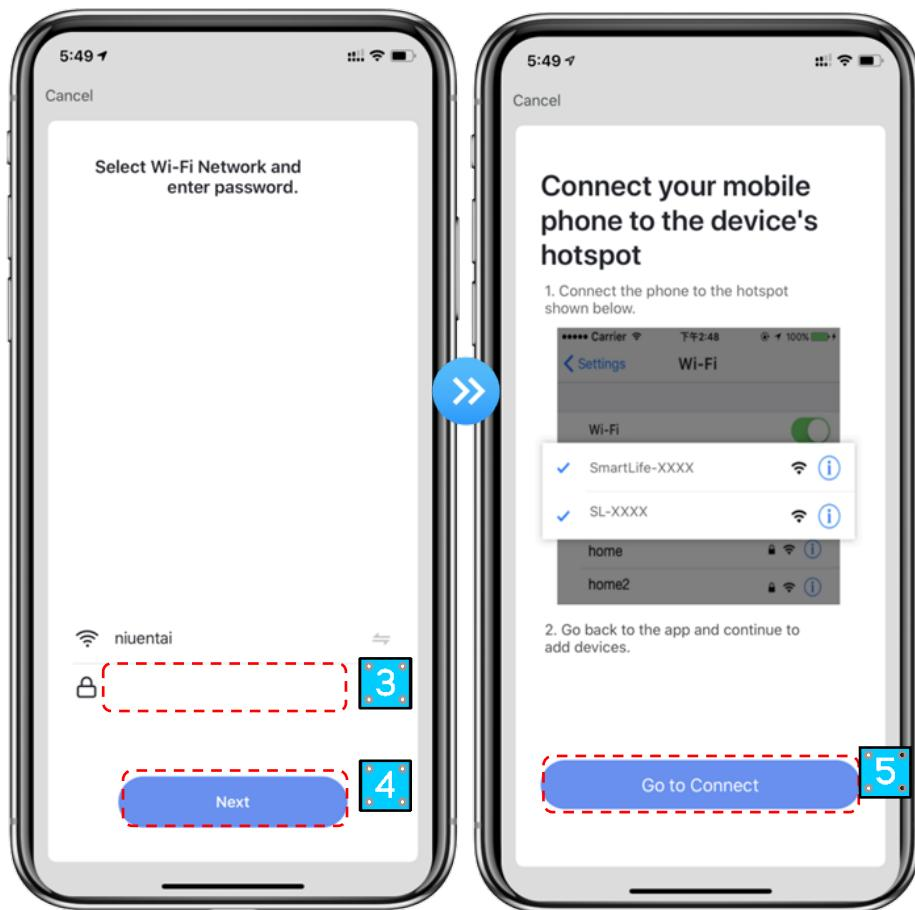
Enter the mobile phone Wi-Fi connection interface, find the “Smart Life\_XXXX” connection, and the APP will automatically enter the device connection status.
